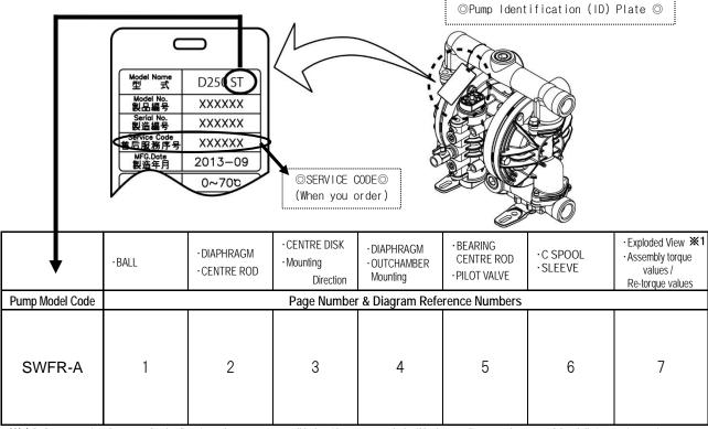
×1) Before operating the pump for the first time please re-torque all bolts. Also re-torque bolts if leaks are discovered as part of the daily inspection regime.
