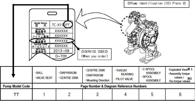
※1)Before operating the pump for the first time please re-torque all bolts. Also re-torque bolts if leaks are discovered as part of the daily inspection regime.
