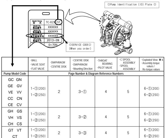
※ 1 )Before operating the pump for the first time please re-torque all bolts. Also re-torque bolts if leaks are discovered as part of the daily inspection regime.
