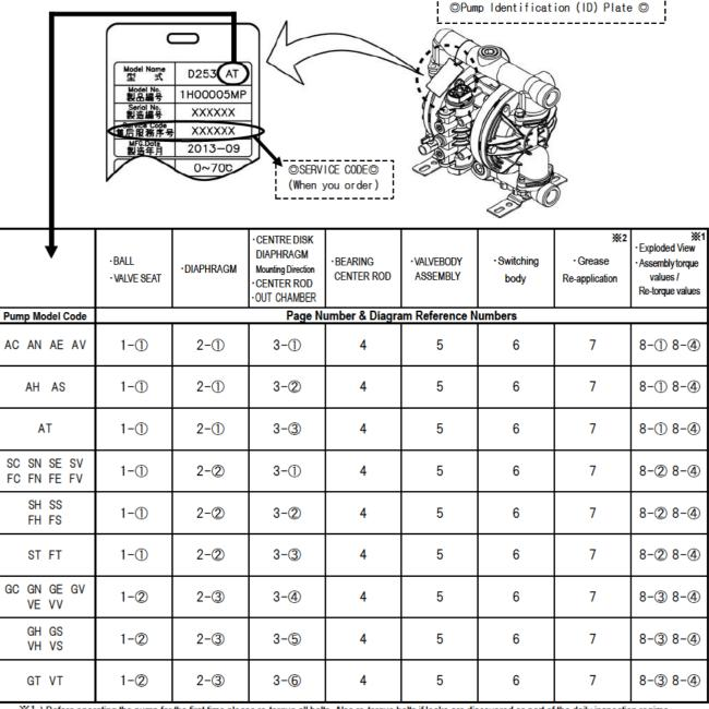
💥 1 ) Before operating the pump for the first time please re-torque all bolts. Also re-torque bolts if leaks are discovered as part of the daily inspection regime.
